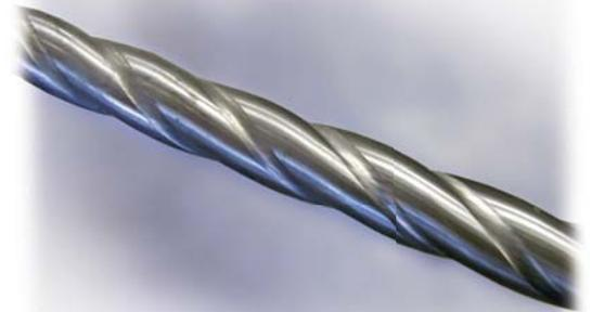
**Corrugation:** The heat exchanger surface is shaped into turbulence-inducing, alternating parallel grooves and ridges to increase heat transfer efficiency. Inducing turbulent flow results in less total surface area required to achieve the desired thermal results. Turbulent flow promotes thorough mixing of the product and even thermal disbursement without compromising product integrity.
